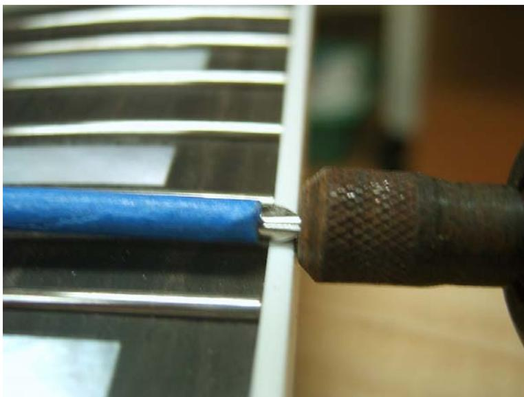
Run the Dremel down the side of the binding with the bit with the taped end resting on the FB and let the exposed portion of the bit remove the bulk of the binding until you got something that looks like this.
