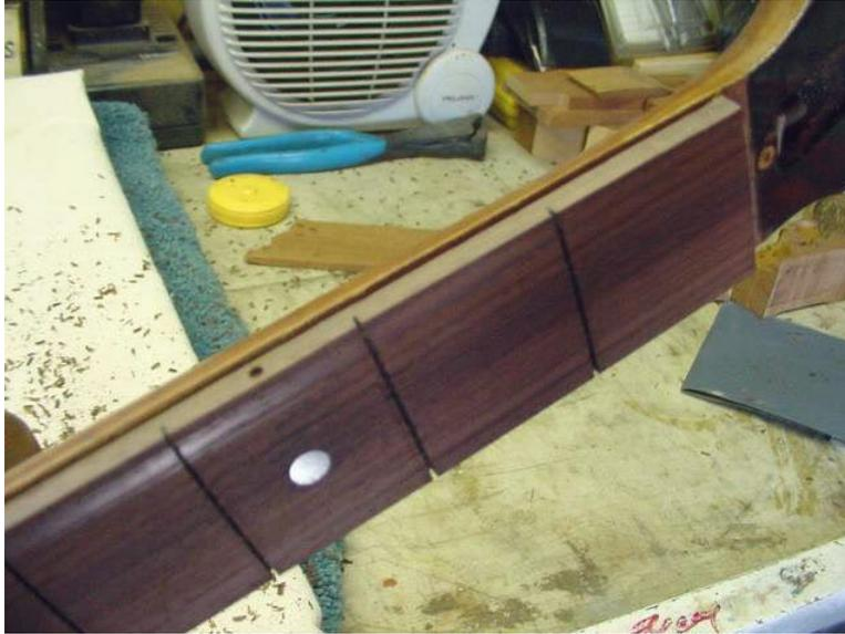
Now you ask, "how did you cut the ledge on the fingerboard that overhangs the body? I used an X-acto razor saw and undercut the fingerboard at the FB/ neck glue joint until the depth of the cut was the same as the depth of the ledge. I used the same saw and following the new edge of the ledge along the top of the FB and cut that until the remaining portion of FB was free. Now if you want to you can also saw off a piece the FB on the end of the neck that's the same thickness of the binding.
