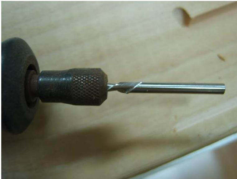
Then I wrap the end of the exposed bit with tape to protect the fretboard. Leave just about 1/8" of the bit exposed...
